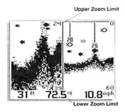
To operate Zoom, press MENU repeatedly until the Zoom menu is on-screen. Three options are available: "Off(Factory Setting), "Auto" (Automatic bottom tracking Zoom), and "Manual" (User controlled Zoom range). Press the DOWN ARROW once to highlight Auto.
